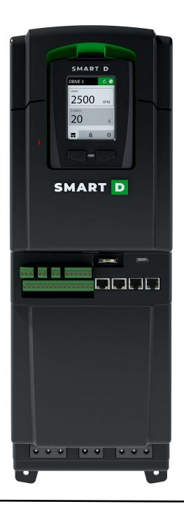
The SmartD *Clean Power* Variable Frequency Drive is a compact AC drive utilizing SmartD's patented own algorithms combined with SiC transistor technology. Producing a clean and pure sine wave to power and control 3-phase AC induction motors has never been easier. The *Clean Power* VFD has essential features built-in for space, wiring and time savings, it eliminates the need for filters on the input and output, and guarantees longer motor lifetime.
