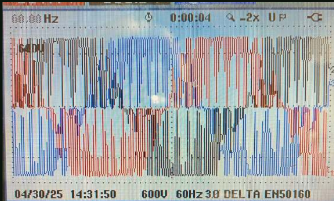
6-pulse VFD — PWM voltage output
